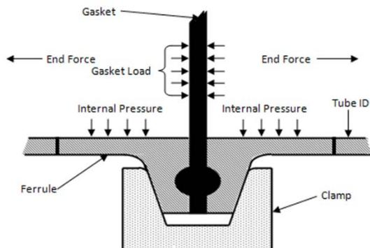
Figure 2 – Forces Acting For and Against Containment
