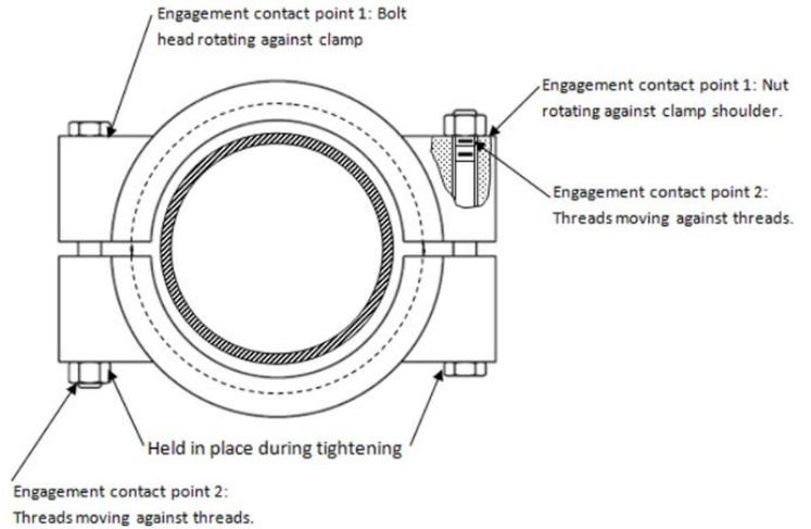
Figure 5 – 2-Bolt High Pressure Clamp Joint Assembly
