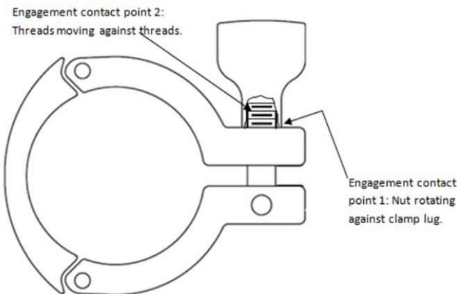
Figure 4 – 3-Piece Double Pin Clamp Joint Assembly
