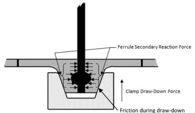
Figure 3 – Forces Acting To Seal the Joint
